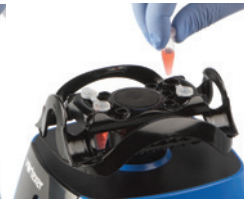
1.5/2.0 mL microfuge tubes x 4 (vertically mounted)
