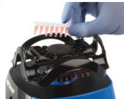
0.2 mL microfuge tubes (strip tubes) x 24 (vertically mounted)
