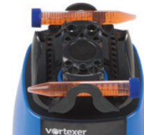
15 mL conical tubes x 2 (horizontally mounted)
