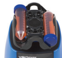
25 mL, 50 mL conical tubes x 2 (horizontally mounted)
